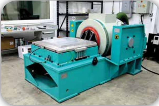
Our dynamics lab features a pneumatic shock machine and three electrodynamic shakers, with the largest being 11,000 lbf and having a three-inch displacement.
